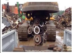
Click on the picture to view how an electromagnet is used to pick up large pieces of metal.
